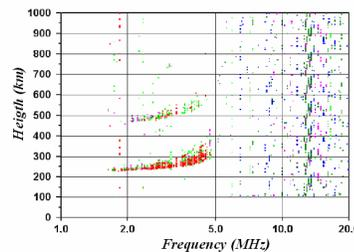
Figure 5: Ionogram with the presence of scattering-type frequency. Adapted from [4].
