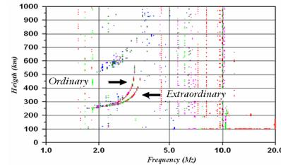
Figure 4: Ionogram with the ordinary and extraordinary traces. Adapted from [4].
