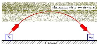
Figure 1: Tilting the path of a wave in an ionized medium.
