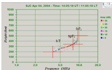
Figure 3: Ionogram showing the virtual height of the layer ( $h'F$ ), maximum or critical frequency ( $f_oF2$ ) and the height in the F layer ( $h_pF2$ ). Adapted from [2].
