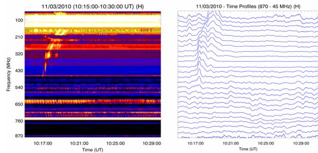
Figure 1: Dynamic spectrum and time profiles (smoothed) of solar split-band type II radio burst recorded on November 3, 2010 ( $\sim 10:17:14$  UT) by CALLISTO-BR spectrometer.
